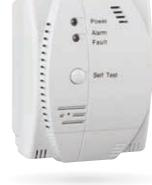
I-9602LW Addressable Gas Detector is used to detect leakage of home use combustible gas (LPG, Natural Gas) in such areas as houses, hotels and apartments. When leakage is detected, the detector will generate high buzzer alert sound, and provide a dry contact to turn exhaust fan, a 12VDC source to switch off the gas valve.
